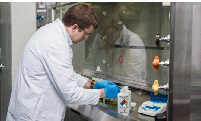
A TerraPower engineer performs chemical experiments in a fume hood. This equipment allows engineers to safely conduct experiments in an air atmosphere.
