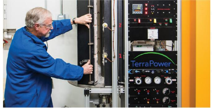
A TerraPower engineer runs a test on a prototype vacuum quench furnace. The full-sized equipment will be used to heat-treat uranium metal to be used in fuel rods.
