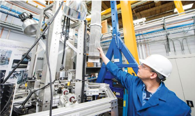
A technician places a full-size test fuel pin bundle in TerraPower's pin duct interaction test apparatus. TerraPower manufactures bench- and full-scale fuel pins and pin bundles for testing in the lab.
