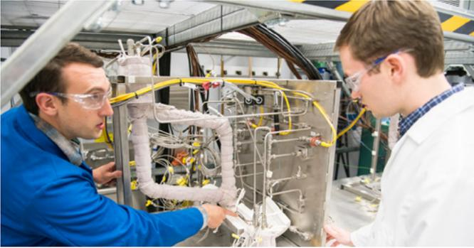
TerraPower rigorously tests molten salts through proprietary loops that demonstrate flow, corrosion and performance at varying temperatures and durations with a variety of structural materials.
